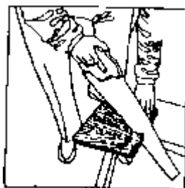
Cutting out the tailgate.
